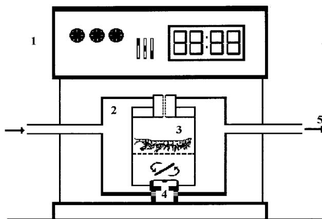
Fig. 2. Respirometer schematic design. (1) Oxygen meter; (2) bath chamber; (3) respirometer chamber and stirrer; (4) electrode; (5) bath water flow
